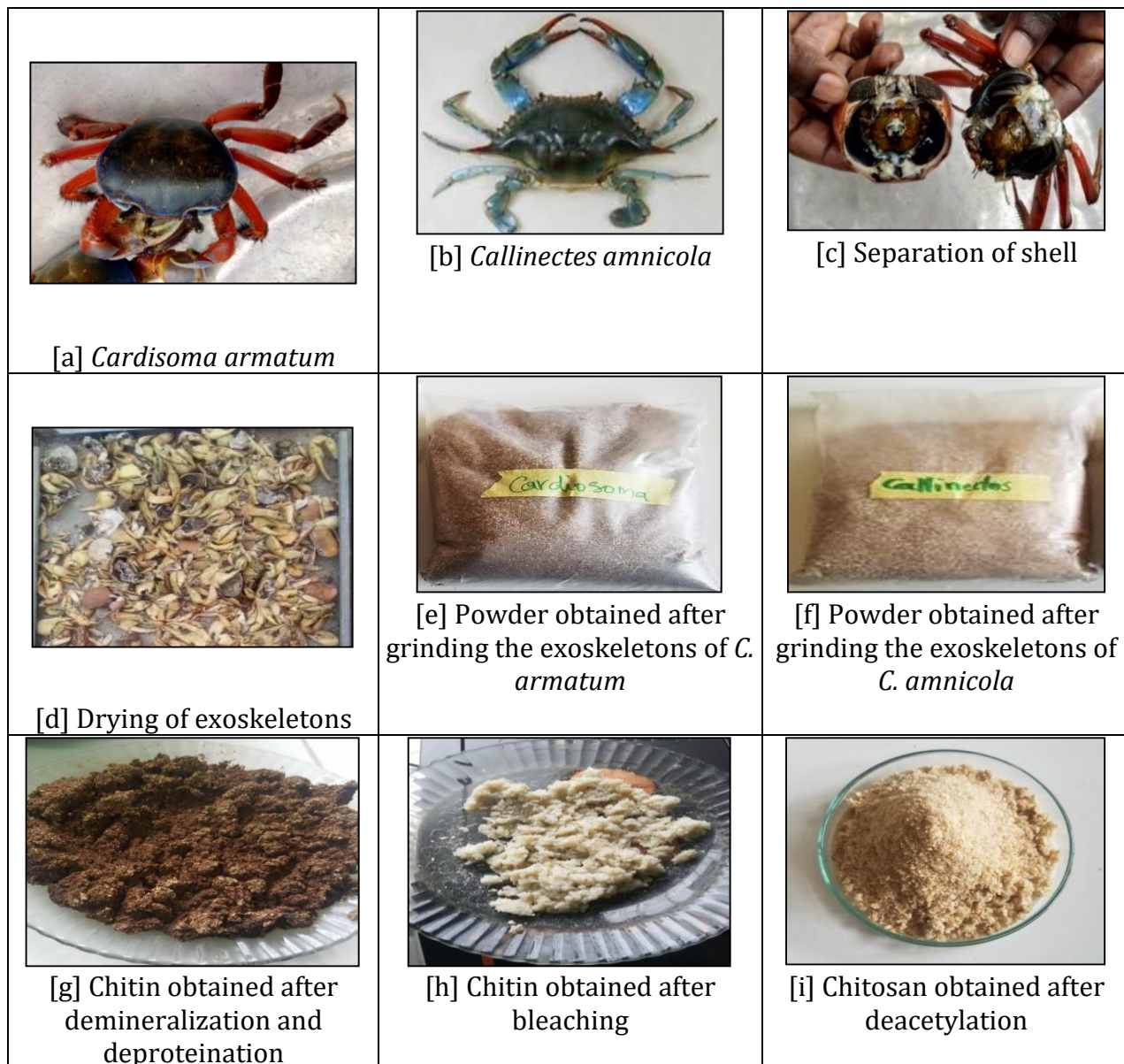
Figure 1. Process of extracting chitin and chitosan from crab shells
