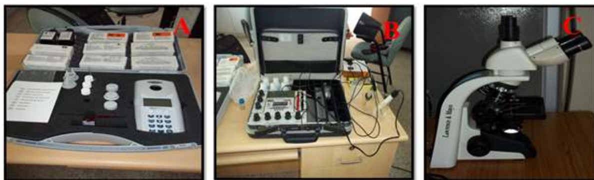
Figure 2 A. Tintometer, B. Soil and Water Analysis kit, C. Lawrence and Mayo Compound microscope
