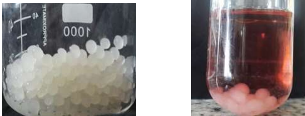
Figure 9 a) Immobilized sodium alginate beads b) Reaction mixture with beads
