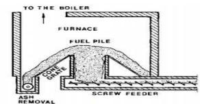
Refractory furnace and underfeed stoker
